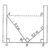
A L-shaped ladder, ABC is wedged in between two pillars AO and DE as shown in the diagram. A and C are the points of contact between the ladder and the pillars while B is the point of contact between the ladder and the ground.
