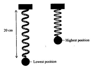
The length of the spring is 20 cm when the weight is at its lowest position and it takes 2 seconds for the weight to move from the lowest to highest position.
