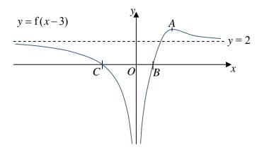
The graph of y = f(x-3) is shown above, where the lines y = 2 and x = 0 are asymptotes to the curve and A(2,3) is a maximum point. The graph also crosses the x-axis at B(1,0) and C(-2,0). On separate diagrams, sketch the graphs of
