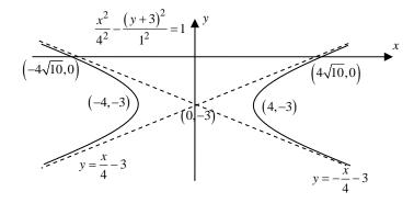
Every line y = mx - 3 passes through (0, -3) and must have a steeper gradient compared to the asymptotes of C.
