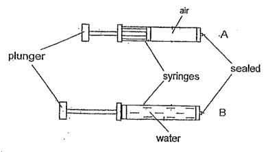
Peter pushed the plunger of syringe A and found that it could be pushed in but plunger of syringe B could not be pushed in at all.
