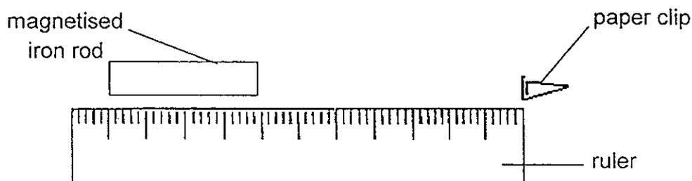
Darren placed the paper clip and magnetized iron rod beside the ruler as shown above. Next, he pushed the iron rod slowly towards the paper clip until the paper clip is attracted to it and recorded the distance. He repeated the above steps with the other 3 magnetised iron rods.
