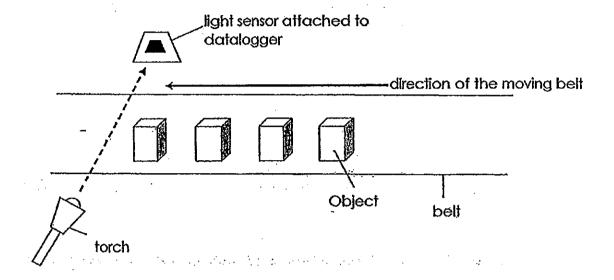
The belt moves at a constant speed. When the object of 1 cm is between the torch and the light sensor, it blocks the light from reaching the light sensor. The data recorded is shown in the graph below.
