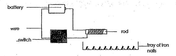
When the switch was-turned on, the rod attracted some of the iron nails in a tray. The number of nails attracted from the tray was recorded in the table below.
