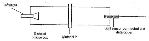
The experiment was repeated with materials Q and R. The amount of light that passed through each material was recorded in the table below.
