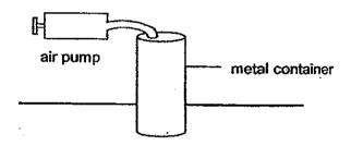
The capacity of the metal container is 400 cm<sup>3</sup>. When the plunger is pushed in completely, 50 cm<sup>3</sup> of air is forced into the metal container. What is the volume of air in the container after the plunger is pushed in once?
