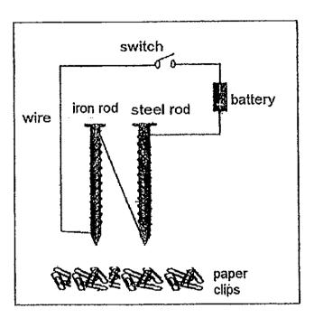
The two rods were placed 5cm above a pile of paper clips which were evenly spread on the table and when the circuit was closed, the number of paper clips attracted to each rod was shown below.
