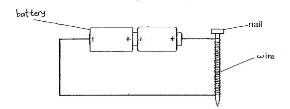
Based on the arrangement above, the electromagnet could pick up 10 paper clips.
