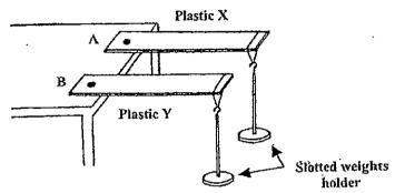
He then added slotted weights, one at a time, to one end of each plastic ruler and recorded the number of slotted weights the rulers could hold before they broke as shown in Diagram 2 below.
