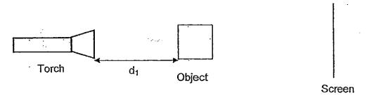
The height of shadow cast on the screen was measured when the torch was switched on. She recorded her results in the table below.
