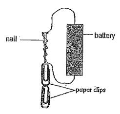
When different numbers of batteries were used and connected by wires, the nail was able to attract different numbers of paper clips. The results are shown in the table below.
