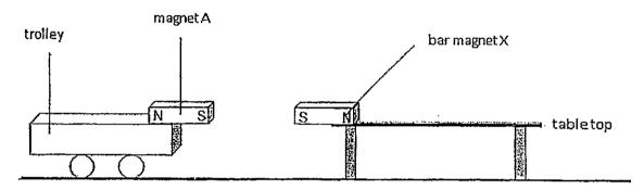
The different magnets were each brought close to the bar magnet X one at a time, till the South poles of the magnets touched each other. The magnets repelled. The trolley was ther let go so that it would travel backwards a distance away from the bar magnet X. The distance that each magnet travelled backwards was measured and recorded in the table below.
