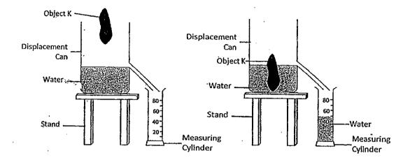
Gary concluded that the volume of object K was 50ml as shown in the measuring cylinder.
