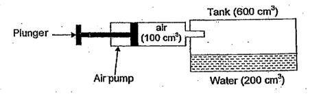
When the plunger of the pump is pushed in completely, 100 cm<sup>3</sup> of air is forced into the tank. What is the volume of air in the tank after the plunger is pushed in?
