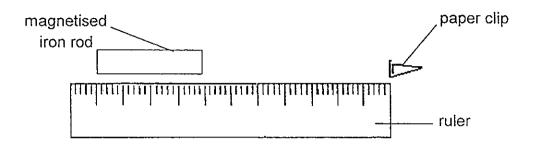
Darren placed the paper clip and magnetized iron rod beside the ruler as shown above. Next, he pushed the iron rod slowly towards the paper clip until the paper clip is attracted to it and recorded the distance. He repeated the above steps with the other 3 magnetised iron rods.
