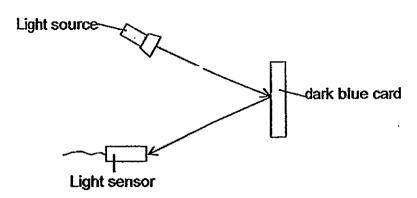
He shone the light source at a dark blue card and used the light sensor to record the amount of light reflected by the card. He repeated his experiment using light blue, dark orange and light orange cards and recorded his results as shown in the graph below.
